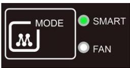
**SMART Mode:** This is designed for maximum convenience and maintains the ideal domestic environment humidity level of 50-55% while saving electricity. This is the default mode and is recommended for most users.
