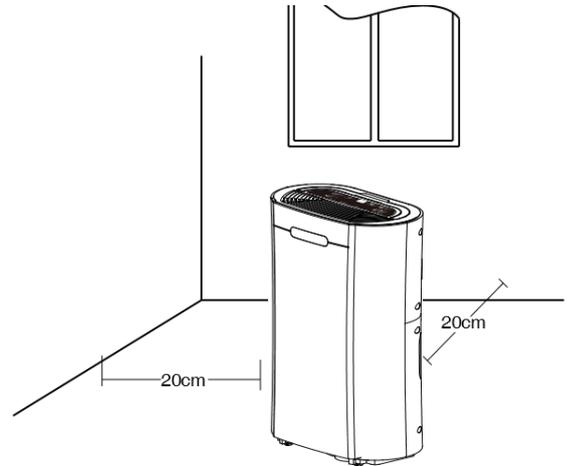
Alternatively, if you have a serious problem in one area you can begin by positioning the dehumidifier there and moving it to a more central location at a later date. For the most effective use, run your dehumidifier with external doors and windows kept closed. Please note the unit should not be placed directly against a radiator or other heat source.
